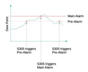
Two alarm levels can be programmed (pre and main alarm), serving an optical indications or separate relay outputs.
