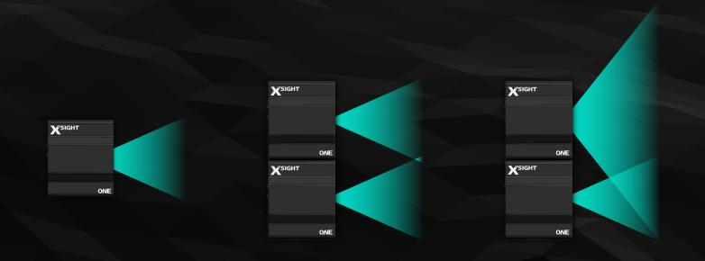
In cases when the field of view of one camera is less than 210 mm, it is not mechanically possible to merge the fields of view. That means the JOINED mode is not applicable.
