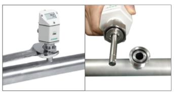
S 420 can be removed from the compressed air or gas line easily for calibration or exchange purposes. The opening can be closed with the optional closing cap (see order information). This is a special advantage as most flow meters on the market require an expensive bypass line in such a case.
