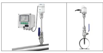
For pipe diameters of DN 50 to DN 300 the insertion type flow meter S 400 is available. This sensor can be inserted into the compressed air or gas pipe through a standard 1/2" ball valve. This allows installations and removal of sensors under pressure without shutting down the air or gas system.
