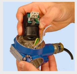
Extract the solenoid coil from the housing, by twisting it gently leading with the top edge.
