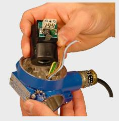
Extract the solenoid coil from the housing, by twisting it gently leading with the top edge.
