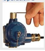
Loosen the security dowel using the setscrew wrench 5
