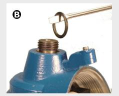
If operation 5 was necessary, carefully extract the O ring from the solenoid coil housing
