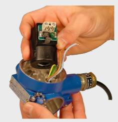
Extract the solenoid coil from the housing, by twisting it gently leading with the top edge.
