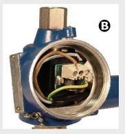
Loosen the terminal board screws and pull out the two power supply Wires (A)
