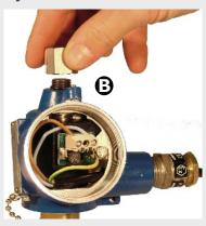
Depending on the model, loosen the hexagonal nut with a 19mm spanner, turning anti-clockwise (A)
