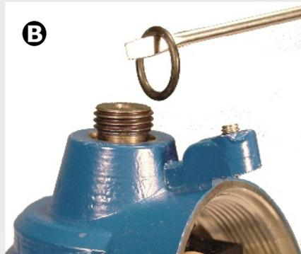
If operation 5 was necessary, carefully extract the O ring from the solenoid coil housing
