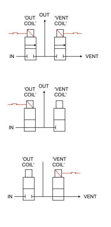
Normal Flow Circuit, both coils energised
