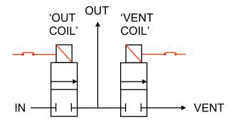
Normal Flow Circuit, both coils energised
