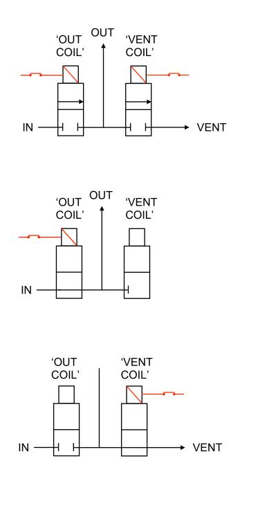
Normal Flow Circuit, both coils energised
